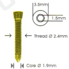
SAFETY LOCK SCREW \varnothing 2.4MM SELF TAPPING
