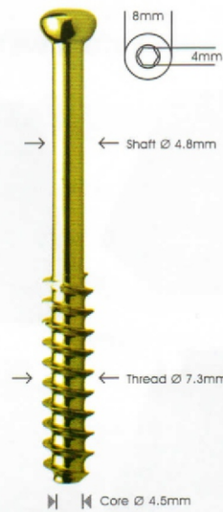
CANCELLOUS CANNULATED SCREW Ø 7.3MM 32MM THREAD
